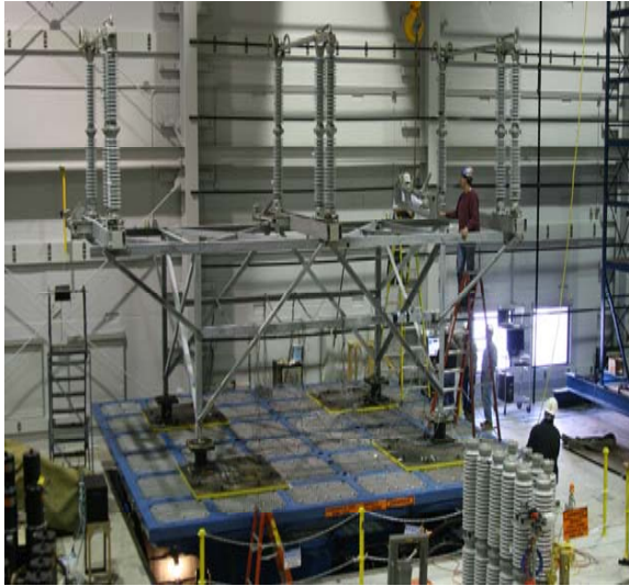
Seismic Qualification and Fragility Tests of a 230KV-3 Phase Switch Assembly
