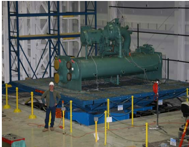
Seismic Fragility Tests of a Centrifugal Liquid Chiller and Restraint System
