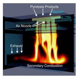
right is from a recent analysis performed by Professor DesJardin in support of this project. It depicts turbulent combustion of pyrolysis products mixed with fresh air provided by the inlet small inlet nozzles of the boiler.
