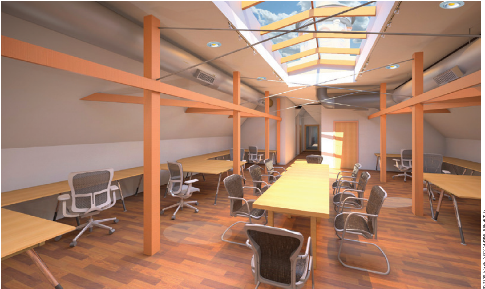
Exposed wooden trusses and skylights will brighten up the reclaimed fourth-floor attic spaces.
