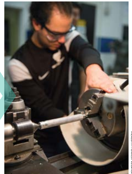
A student uses a lathe to fabricate a metal hammer in Engineering Machine Shop.
